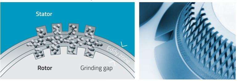
The principle of the PUC colloid mill is based on a rotor/stator system. In a stator tailored to the product to be processed with suitable teeth there is a rotor which has teeth of its own. As a result of the different conicity of the toothed tapered surfaces of the roter and the stator a ring gap which becomes more and more narrow is produced in the direction of flow towards the outfeed cross section.
