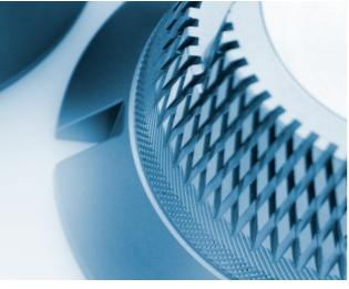
The principle of the PUC colloid mill is based on a rotor/stator system. In a stator tailored to the product to be processed with suitable teeth there is a rotor which has teeth of its own. As a result of the different conicity of the toothed tapered surfaces of the roter and the stator a ring gap which becomes more and more narrow is produced in the direction of flow towards the outfeed cross section.
